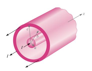
In the coax line, we have two concentric *solid* conductors that carry equal and opposite currents, *I*.
